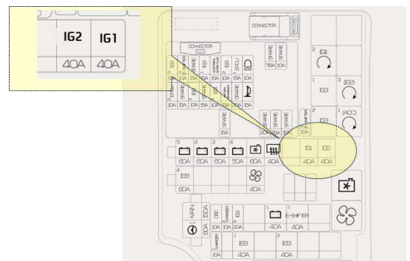
motor compartment fuse box
